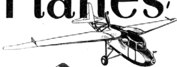
SKYCAR (Above).—With the passengers' cabin in the nose and the airscrew revolving in an open framework at the rear, this is the "Stout Sky-car," designed as an aerial runabout.
